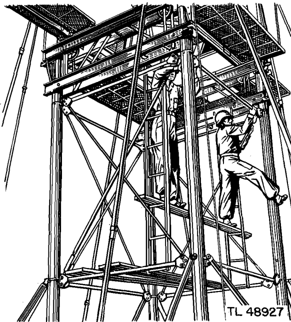
Figure 2-29. Use of ladder sections in installing braces.
